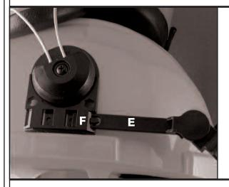
Checking that the arms are uppermost as shown, install the face guard support saddle by locating the arms (E) into the slots on the ear defenders (F). Push both arms until they click into place in the locking cut-outs (F) as shown. Ensure both arms are in the same cut-outs.
